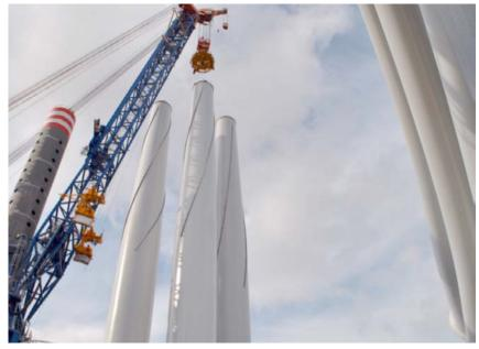
Here we can see nine Siemens B75 blades loaded in to the blade rack and secured ready for transport. The B75 blade, which measures 75 metres in length, is the world's largest fiberglass component cast in one piece.
