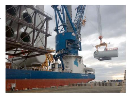
88 metre turbine towers being secured to the deck of the Sea Challenger. The spiral wraps seen on the towers are temporarily fitted to reduce vortex forming (which could cause instability) above the towers during transportation.
