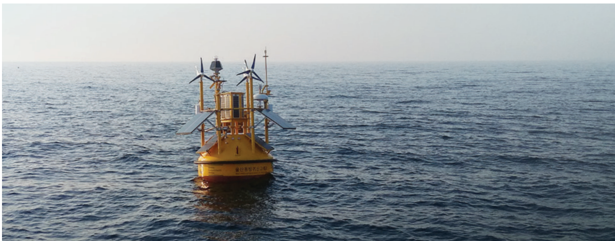
Right: Korea's first floating LiDAR system
